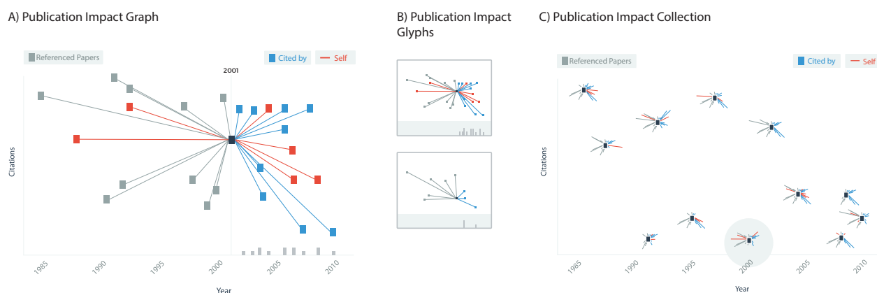
Figure 1: A) A publication impact graph uses time on the X axis, and citations on the Y axis to visualise a publication in context with the references for that paper, and the papers that have cited it. B) Glyphs representations are a more compact version of A) with the citation histogram distinguish by its own section in the glyph. C) Visualise the publication space for an author, institution, or subject area by placing many impact glyphs in 2D space. Citation lines are truncated and expandable with interaction.
