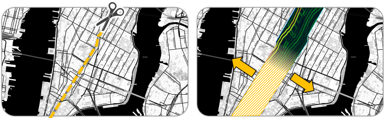
Figure 1: Illustration of the principle of SpaceCuts: By cutting a map along a selected feature, for example Broadway in New York (left), the resulting map parts can be pulled apart to create additional space for visualizations. The yellow shaded area illustrates the gained space (right) and an example how it could be used for an arbitrary visualization in the upper half.
