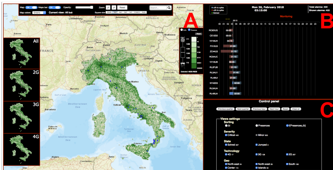
Figure 1: Overview of the visual analytics system for failures analysis that includes three main views: the geographical analysis environment (A), for identification of zones with failures, the temporal analysis environment (B), for estimating the failures impact and prioritize interventions, and the analysis control panel (C), to parametrize the analysis.
