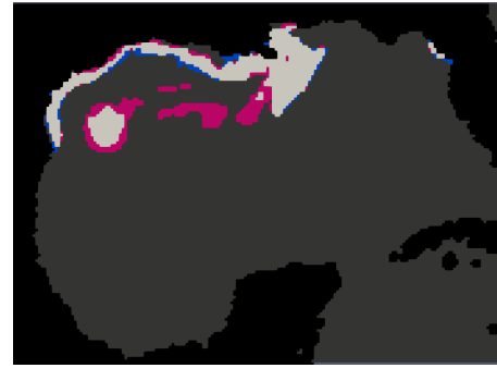
Figure 9: Quantitative analysis of the evolution of the nutrients for statistical evaluation. The areas dominated by advection are light grey, upwelling pink, downwelling blue, and neither black.
