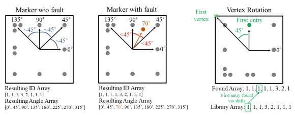
Figure 5: Left is a tile without detection fault. The entries of its ID array are derived from the single groups of dots. Here, a single dot refers to an entry of 1, two dots to an entry of 2 and so on. The angle difference to the next groups should be the same. The middle shows a tile with detection fault which results in a smaller angle to the next dot groups. **Right**, the vertex calculation and rotation calculation is depicted.
