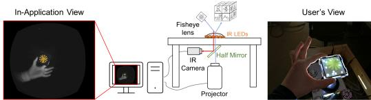
Figure 2: System overview of the axis aligned projector-camera setup, the user's view and the in-application view.
