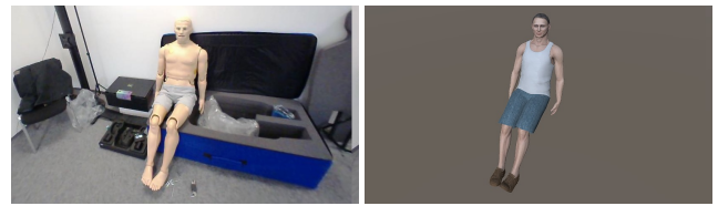
Figure 2: Camera image of the medical manikin (left) and the corresponding HMD view of the virtual patient after body pose estimation using keypoint detection (right).
