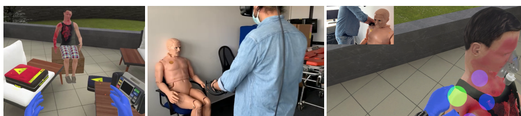
Figure 1: Estimating the pose of a medical manikin can be used for haptic support in medical training.
