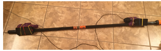
Figure 1: The apparatus has a Razer Hydra controller on each end with the Sony Xperia ZR on the right and the Samsung Galaxy S4 on the left.
