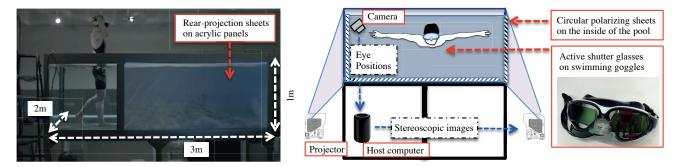
**Figure 3:** The system configuration of AquaCAVE: Stereoscopic images are projected on each wall of the swimming pool. The user wears 3D glasses on swimming goggles in the pool, and the head position is tracked for configuring an immersive environment. The inside of the pool is coated with circular polarizing sheets for a constantly clear view, stable head tracking, and reflection reduction.
