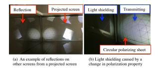
**Figure 5:** *Reflection reduction by circular polarization.*
