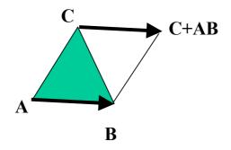
Fig 20: Parallelogram used for predicting a vertex.
