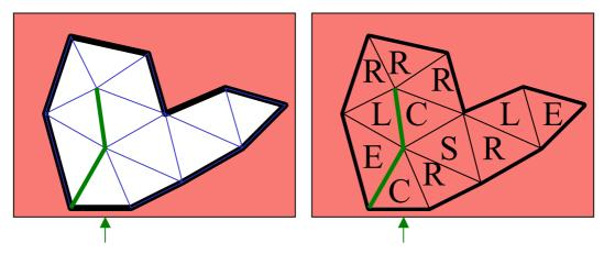
Fig 10: Typical ending Edgebreaker sequence, producing the clers stream CRSRLECRRRLE
