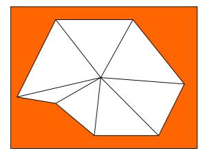
Fig 18: Filling the hole with a dummy vertex.
