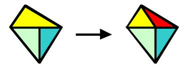
Fig 4: Splitting a triangle to remove a T-junction
