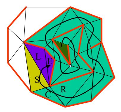
**Fig 9:** A more complex Edgebreaker beginning producing the *clers* stream CCCRCCCRCCCRRLCCCRCSLE
