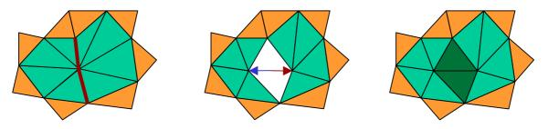
Fig 21: Vertex insertion (the inverse of an edge collapse).
