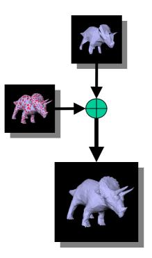
Fig 24: Progressive transmission (crude model plus upgrades)
