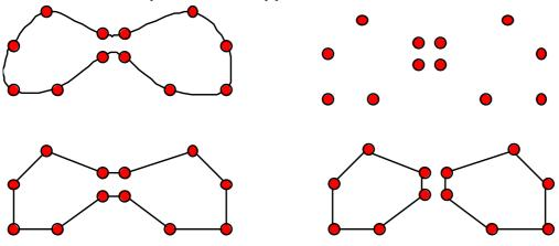
Fig 2: The interpolation of a set of sample points may have the wrong smoothness or connectivity.
