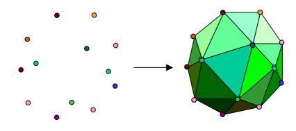
Fig 1: The interpolation of a set of sample points by a triangle mesh
