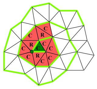
Fig 7: Typical starting Edgebreaker sequence, producing the clers stream CCCCCRCCRCRC
