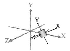
b. New coordinate system, scaled by half, rotated 30.0 degrees around Z, and translated 2.0 units in X
