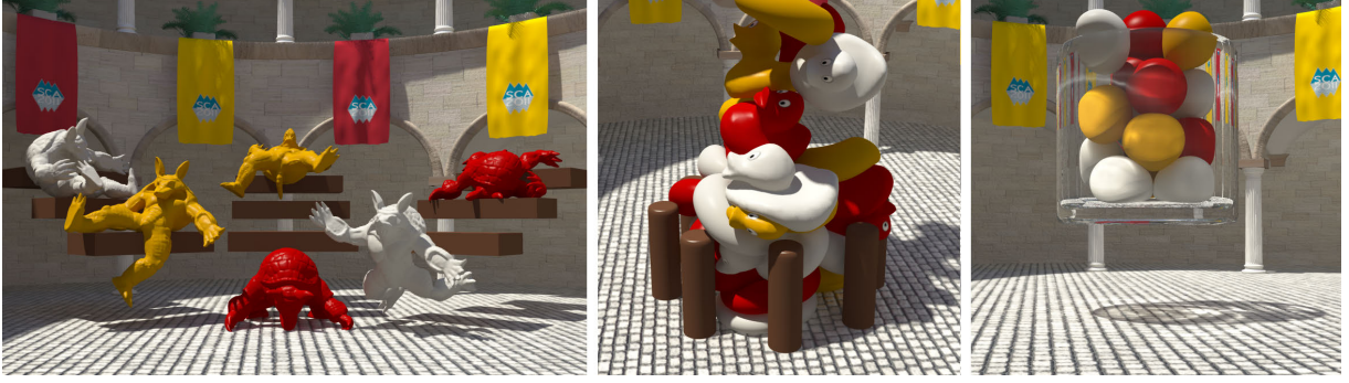
Figure 23: Robust and volume-conserving deformations using shape matching. Armadillos (32442 particles total), 20 ducks and 20 tori (21280 particles total) and 20 balls (7640 particles total) were simulated in real-time on a GPU.
