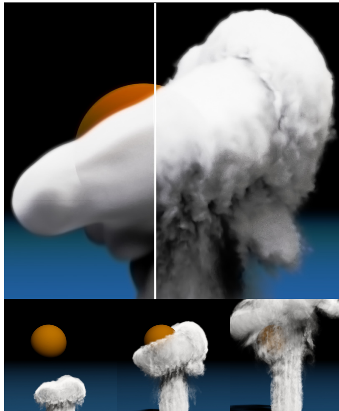
Figure 4.4: Flow around a sphere with grid-based densities. The low resolution simulation is shown in the left half of the top image. Wavelet turbulence synthesized a 400^3 grid from a 50^3 grid. Each frame took an of average 30 seconds on a four core workstation.
