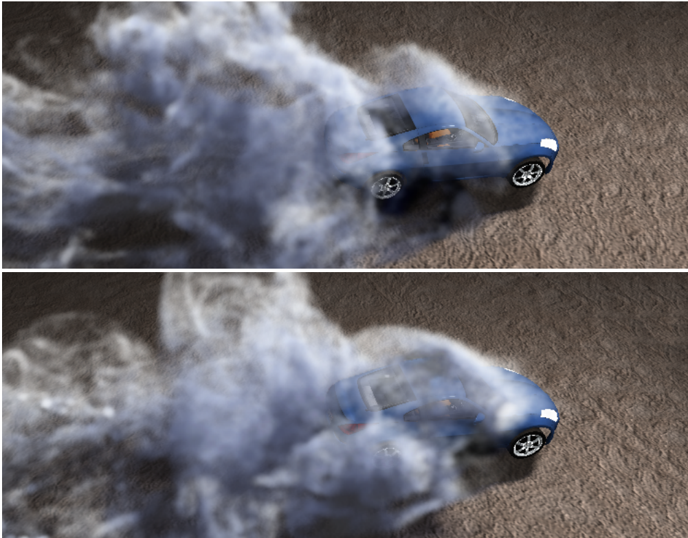
Figure 4.11: The wake behind a car is simulated with 1M particles. Our method (top) and the reference high-resolution solver (bottom) show similar small-scale details.
