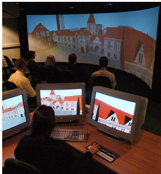
Figure 2: A large-scale, front projected, semi-immersive virtual environment.
