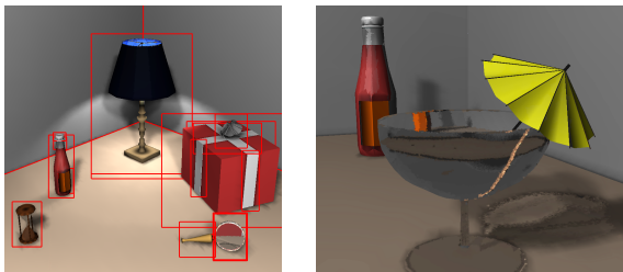
Figure 13: Left: the object structure of a sample scene. Each red box corresponds to one object that shares one corrective texture. Right: a resulting rendering exhibiting reflections, refractions, and a caustic. Images courtesy of Marc Stamminger.
