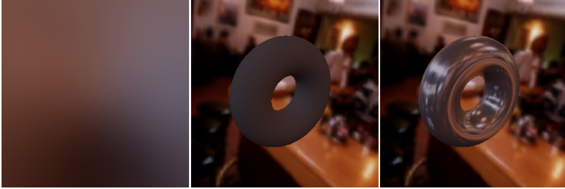
Figure 6: Left: diffusely prefiltered environment map of the cafe scene. Center: diffusely illuminated torus. Right: same torus illuminated with both a diffuse and a mirror term.
