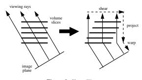
Figure 9: Shear Warp
