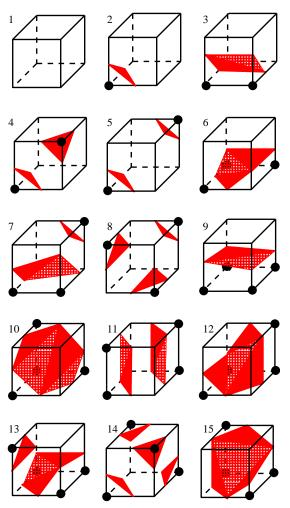
Figure 3: The 15 Marching Cubes configurations
