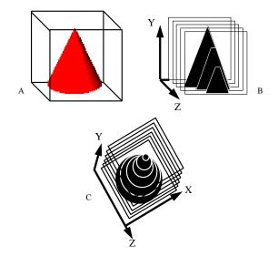
**Figure 10:** Using 2D textures for Volume Rendering: A) Represents a volume of binary data containing a solid cone; b) shows the volume being sliced in the XY plane with a texture map being pasted onto each rectangle; c) shows the same process, but in the XZ plane
