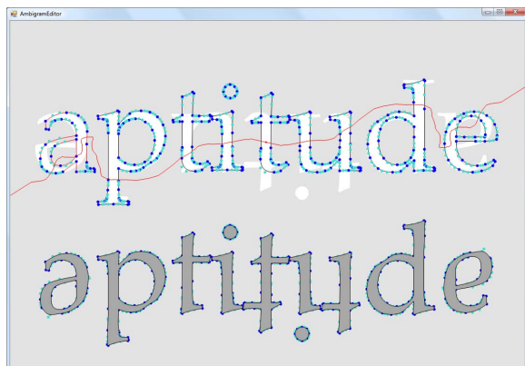
Figure 1: The ambigram editor offers standard editing functions but enforces symmetry. It cuts the shapes along a path drawn by the user, mirrors them and connects the mirrored ones to the original ones with adjustably soft transitions. The input is displayed in the top half, the output in the lower half.
