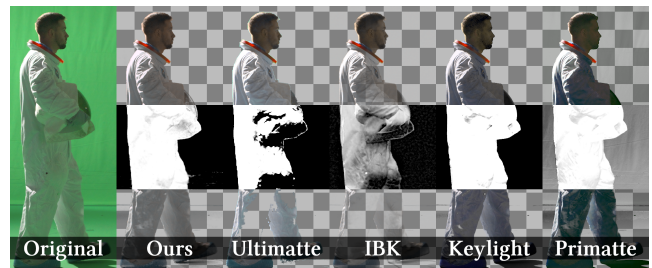
Figure 1: This footage of an astronaut walking contains tremendous amounts of screen spill from the floor and walls. Our method achieves the best result. Note the neutral spill suppression on the astronaut's suit, a perfectly transparent \alpha = 0 background as seen in the center strip, edge detail retention, and limited holes in the foreground. Footage courtesy ActionVFX.
