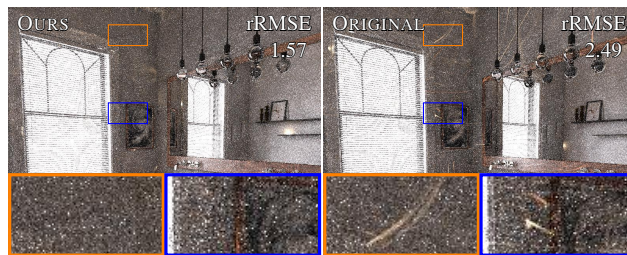
Figure 5: Equal-sample (200 mpp) rendering of contemporary-bathroom. The original implementation produces sharp features that are notoriously difficult to denoise whereas our approach presents far fewer of these artifacts, and a better rRMSE.
