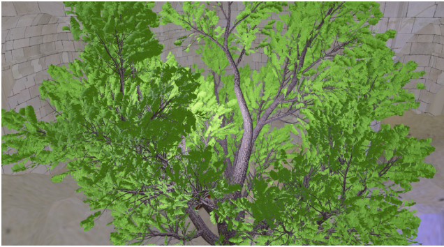
Figure 6: Complex scene for memory requirements. It needs 115.31 MB memory for 8x and 75.01 MB for 4x anti-aliasing. In the 8x case it is even smaller than the memory requirements of the traditional 4x MSAA implementation.
