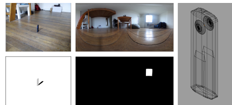
Figure 2: Input data left column: local scene and masks of the main object and its shadow, corresponding to the light in the EM (middle column). Right: 3D geometry of the main object (i.e., 360° camera) present in the local scene.
