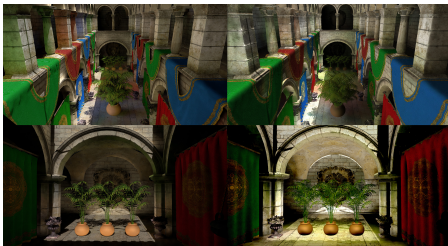
Figure 1: The Crytek Sponza Scene with two sets of images, the left of each pair using NVIDIA's DXR and the right using a Voxel-Based ray marching technique.
