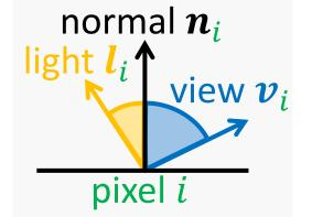
$w_i = \min(m_i, \max(0, \langle n_i, l_i \rangle \cdot \langle n_i, v_i \rangle))$  $m_i \in \{0,1\}$ : visibility (from light and view)
