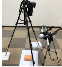
Figure 4: Experimental setting for projection mapping using an abdominal model
