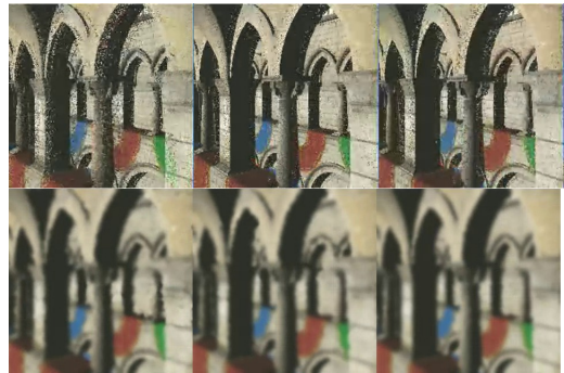
Figure 2: Comparing our adaptive frameless rendering prototype (bottom) to a non-adaptive frameless renderer (top). The result of using differing numbers of sampling threads are shown from left to right: 256x64, 256x128, 256x256
