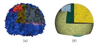
**Figure 3:** Insertion into a badly shaped THex mesh. In (a), the geometric model is captured; in (b), the surface classification is shown and projection and smoothing was applied.
