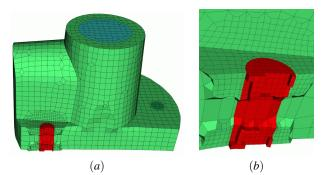
Figure 2: The initial mesh is refined to insert the red cylinder. In (a) a global view is shown; in (b) the refinement area.
