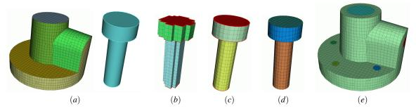
**Figure 1:** Insertion of a geometric element into an existing hexahedral mesh. In (a), the reference mesh M and the geometric element  $G_2$  to be inserted; in (b), cells of M that will be in  $G_2$  are selected and curves and surfaces classification is done; in (c), nodes are projected onto  $G_2$  while a sheet is inserted to improve mesh quality in (d). In (e), several imprintings have been performed to enrich the reference mesh.
