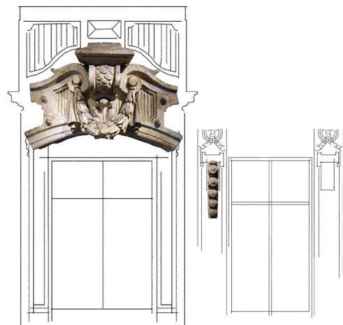
Figure 8: Spatial collage of 3D scanned monument superimposed over 2D drawing showing the overall organization of the wall assembly. (Julia Wiśniewska and Adam Miziołek, 2023)
