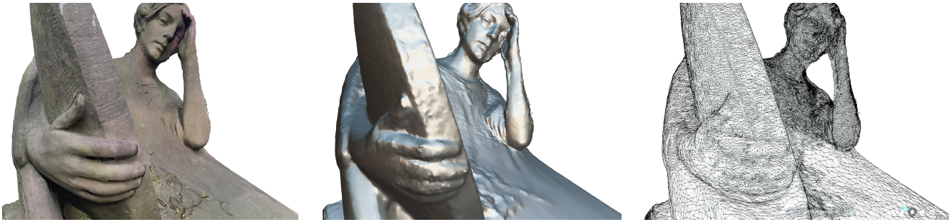
Figure 6: The closeup of the Orłowski's tombstone shows the level of detail and textures (left), the shaded model shows the quality of the surfaces (center), and the wireframe model shows the density of triangular mesh (right) (Agnieszka Jędruszek and Łukasz Polewczyk, 2023).
