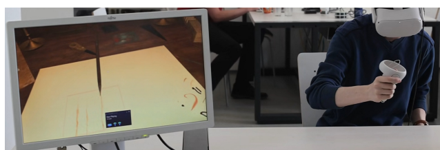
Figure 8: Drawing using 1st variant, where drawing occurs when the virtual pen touches the virtual paper in the scene. The participant holds the controller in the air and draws with the virtual pen without haptic feedback.
