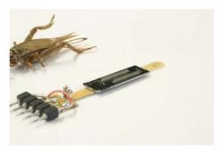
**Figure 1:** The cricket and the bio-inspired MEMS hair array sensor.
