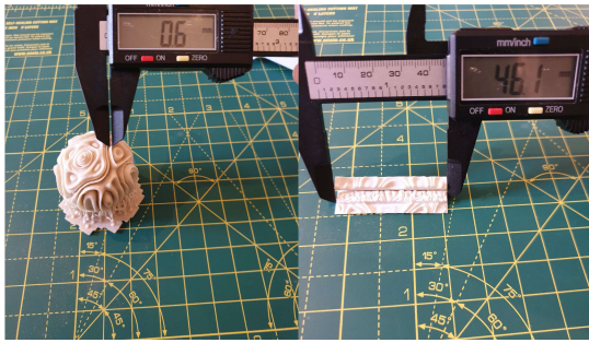
Figure 16: 3D print outputs using Chladni texture: on the left, we demonstrate a Chladni texture application on a sphere, and on the right are 3D prints of three patterns on plane slices.
