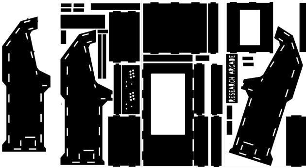
Figure 2: The Research Arcade Machines were designed to be cut by a CNC router
