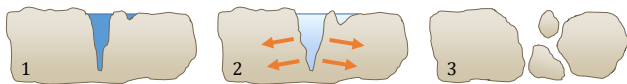
Figure 2: Mechanical erosion produced by freeze-thaw cycles. Water infiltrates into fractures of the rock (1). When it freezes, its volume expands and pressures on the fracture walls, enlarging the fracture (2). Rising temperatures will melt the ice, repeating the cycle and eroding the rock (3).
