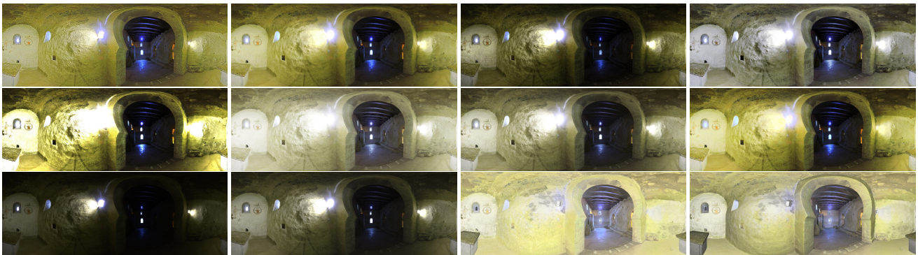
Figure 5: Comparison with common tone mapping operators. We used the default parameters recommended in Luminance HDR 2.6.0 software. First row: Ashikhmin [Ash02], Drago et al. [DMAC03], Fattal et al. [FLW02] and Ferradance et al. [FBPC11]. Second row: Lischinski et al. [LFUS06], Mai et al. [MMM*10], Mantiuk et al. [MDK08] and Reinhard et al. [RSSF02]. Third row: Reinhard et al. [RD05], Van Hateren [VH06] and our approach (unlit/relit).
