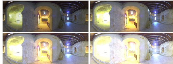
Figure 2: LDR images with increasing gain factors (1, 2.5, 5, 10).
