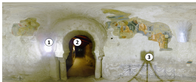
Figure 1: Color artifacts from a sample LiDAR scan: over-exposed areas (1), under-exposed areas (2), and undesirable shadows cast by scanning equipment (3).
