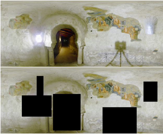
Figure 4: Top: Original color. Bottom: masked regions with low-quality color information. Training tiles will only be generated from non-masked areas.
