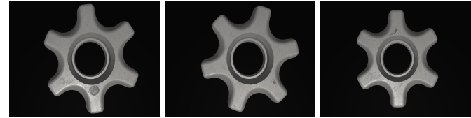
(b) Images of defective components
