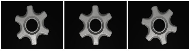
(a) Images of non-defective components
