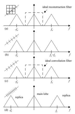
**Figure 3:** *PCVR in frequency space. Step 1: (a) reconstruction of the volume with bandwidth*  $f_v$  *and (b) sampling it into a slice at equal bandwidth*  $f_s=f_v$ ; *Step 2: (c) reconstruction of the slice via convolution with a filter with bandwidth*  $f_s$  *and (d) resampling it into the desired high-resolution grid.*
