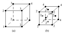
**Figure 8:** (a) Cubic cartesian (CC) cell in frequency space, (b) Face centered cartesian (FCC) cell in frequency space. The dot labeled '1' marks the location of the main spectrum. The dots labeled '2' mark the 1-neighbors (the neighbors with distance=1), the dots labeled '2' mark the  $\sqrt{2}$  neighbors, while the dots labeled '3' mark the  $\sqrt{3}$  -neighbors.
