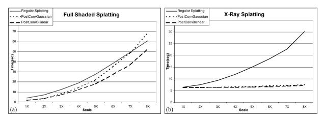
**Figure 10:** Impact of PCVR on our splating pipeline for: (a) Full Volume rendering, (b) X-Ray Splatting. The graphs show time to render in seconds for scales of 1X to 8X.
