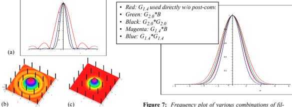
**Figure 5:** (a) Radial profile of the 2D frequency responses for the radially symmetric box (red), linear (blue), and Gaussian (black) filters. (b) 2D plot of the frequency response of the linear filter, the black bars denote the DC locations of the signal replicas. (c) 2D plot of the frequency response of the Gaussian filter.
