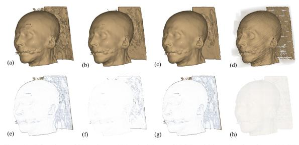
**Figure 11:** Full rendering of CT Head using: (a) Regular Splatting, (b) PCVR with bilinear Post Convolution, (c) PCVR with gaussian Post Convolution, (d) PCVR with Bilinear Spreading (pre-convolution). (e),(f),(g): Difference Images of (a-b), (b-c), (a-c). (h) PCVR without the Post Convolution, to better demonstrate the process.
