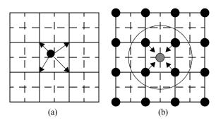
**Figure 1:** Two-phase splatting for magnification=2: (a) splatting of a voxel into a (low-resolution) grid at volume resolution, (b) post-convolution of the low-resolution grid samples to give the high resolution grid samples.
