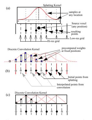
**Figure 9:** Overview of the PCVR in our splatting pipeline: (a) splatting of a voxel into a (low-resolution) grid at volume resolution, (b) post-convolution of the low-resolution grid samples to give the high resolution grid samples, using Gaussian kernel, (c) using a linear bilinear filter (shown for 1D)
