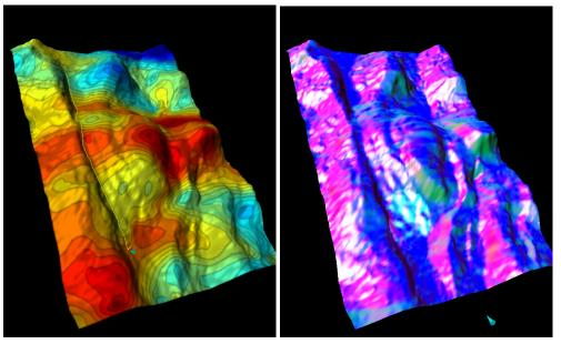
Figure 6. Depiction of gravity data texture-mapped onto the Figure 7. Depiction of the seafloor data with curvature seafloor.
