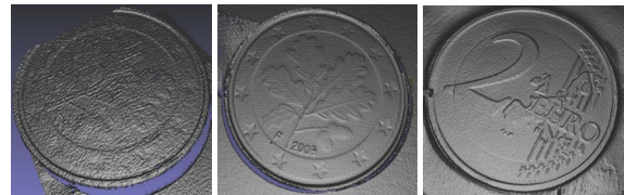
Figure 8: Reconstruction of a 5 cent euro coin with no treatment (left) and with prior application of white paint (middle); reconstruction of 2 euro coin using modeling clay (right).
