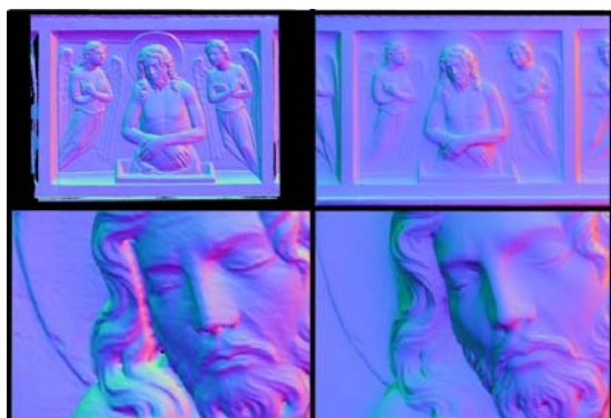
Figure 4: Comparison between the normal maps of the 3D scanning and the PTM: full model and particular.
