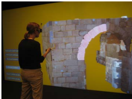
Figure 8: Immersive visualization of part of the castle wall using a 6x2.5m 2 rear projected stereo wall.
