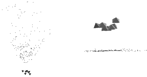
Figure 9: The camera calibration of the images and a set of 3D points, representing the scene, retrieved by our structure and motion algorithm. Both a top and a side view are shown. The planar nature of the scene can clearly be recognized.
