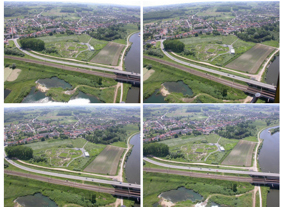
Figure 8: Four of the seven images that served as input for one structure and motion process. The images were taken during different passes of the helicopter and are selected automatically using the matrix in fig. 7.
