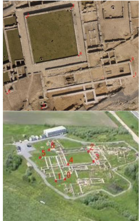
Figure 11: Pose estimation with manual interaction. Corresponding points (red) are indicated both on the ortho-photo (top) and on the image taken from the helicopter (bottom).
