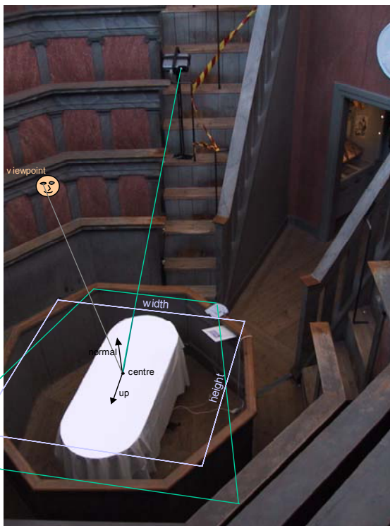
Figure 2: The historic projection environment (left). Graphical sketch of the relationship between on-screen projected coordinates and pre-distorted coordinates in image space (right).
