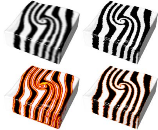
Figure 10: Left: initial points (12k). Right: upsampled points (140k). Bottom row: smoothing related to the original texture.
