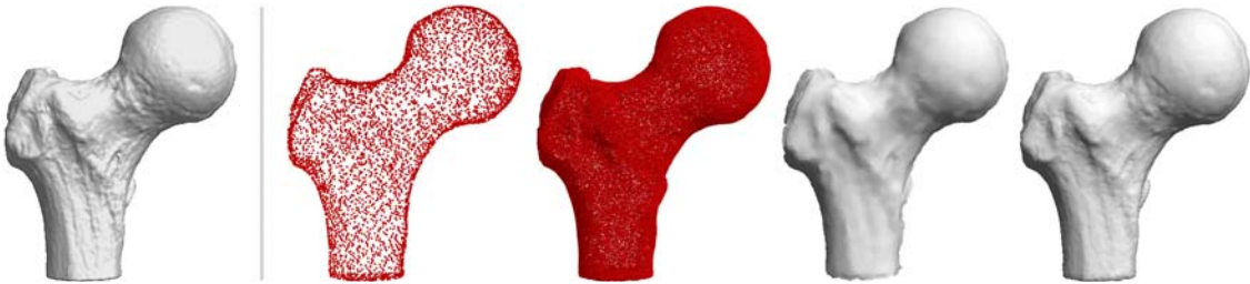
Figure 11: From left to right: splatted surface of the original point model (140k), initial points (9k) randomly chosen from the original model, upsampled points (50k), splatted surface of the initial point set, splatted surface of the upsampled point set.
