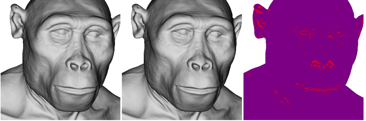
Figure 3: A comparison of using the direction of smallest co-variance \mathbf{n} and \nabla f for image synthesis. The images have been generated by ray tracing the surface. The left image is shaded using \mathbf{n} and appears slightly smoothed in areas of high complexity as compared to the center image, which has been generated using \nabla f for shading. The right images illustrates the difference by color coding the scalar product \mathbf{n}^T \nabla f / \|\nabla f\| .
