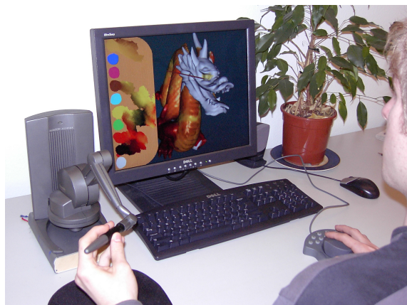
Figure 1: The user interface. The brush is controlled via a PHANToM Desktop haptic device. The object can be rotated using a SpaceMouse.
