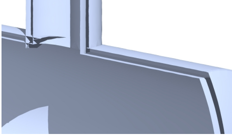
Figure 7: Part surface (cf. Fig. 6) and the oriented envelope. Here trimming is necessary.
