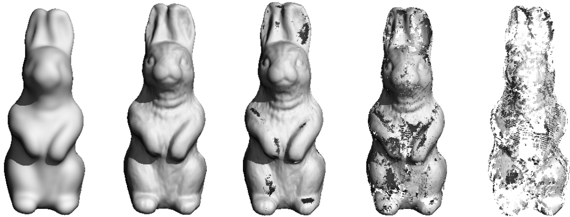
Figure 5: Cyberware's Rabbit, consisting of 67,038 points, ray traced to images with 200x400 pixels using different Gaussian weighting functions. If the radius of the weights becomes too small, the surface is effectively undersampled w.r.t. to the weighting, thus, illustrating the effect of insufficient sampling density. Values for the parameter h relative to the objects diameter from left to right: 1.7%, 0.375%, 0.22%, 0.19%, 0.17%.
