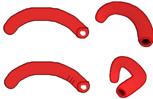
Figure 3: Input sketches (left) and inferred 3D shapes (right) illustrating uniform curvature, versus the use of hatching for indicating the highly curved region.
