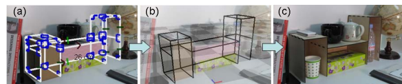
Figure 1: (a) Photo and 2D user sketch of a new and personalized desktop organizer. (b) 3D virtual model visualized and adjusted before production of actual object. (c) New real-world object fits well with other existing objects.
