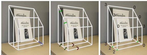
Figure 5: Left: Selecting edges with the mouse cursor. Middle: Three groups (each with different color) of two annotated lines. Green dash symbols are for same length lines and red arrows are for parallel lines. Right: Green highlighted vertices are ground vertices. Each vertex is labeled with the number of dimensions used in the full optimization. The total number of dimensions is reduced from 36 to 18.
