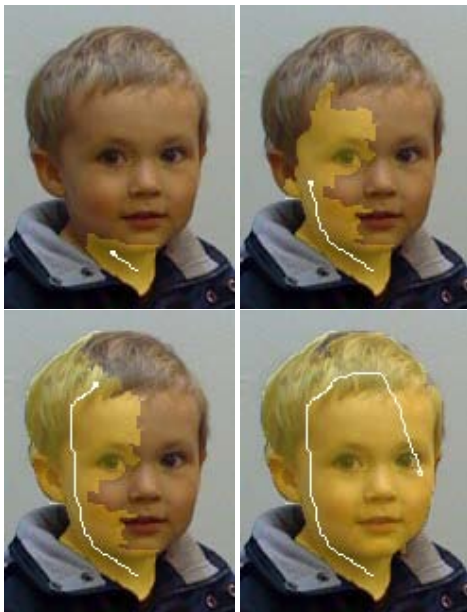
Figure 3: Selection example. Here we are selecting a person and starting with the face. This example uses the length-based stroke method. As the stroke progresses, patches are chosen from increasingly higher levels of the pyramid.
