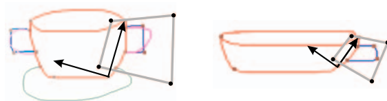
Figure 5: Transformation of the bounding polygon for the right-cup handle. The template is shown on the left, and a sketch on the right. The right-hand edge of the cup-body template serves as the parent edge for this part.
